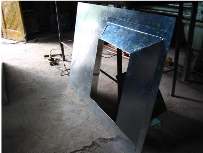
The back cover of the oven has to be adapted for the receiver window.
