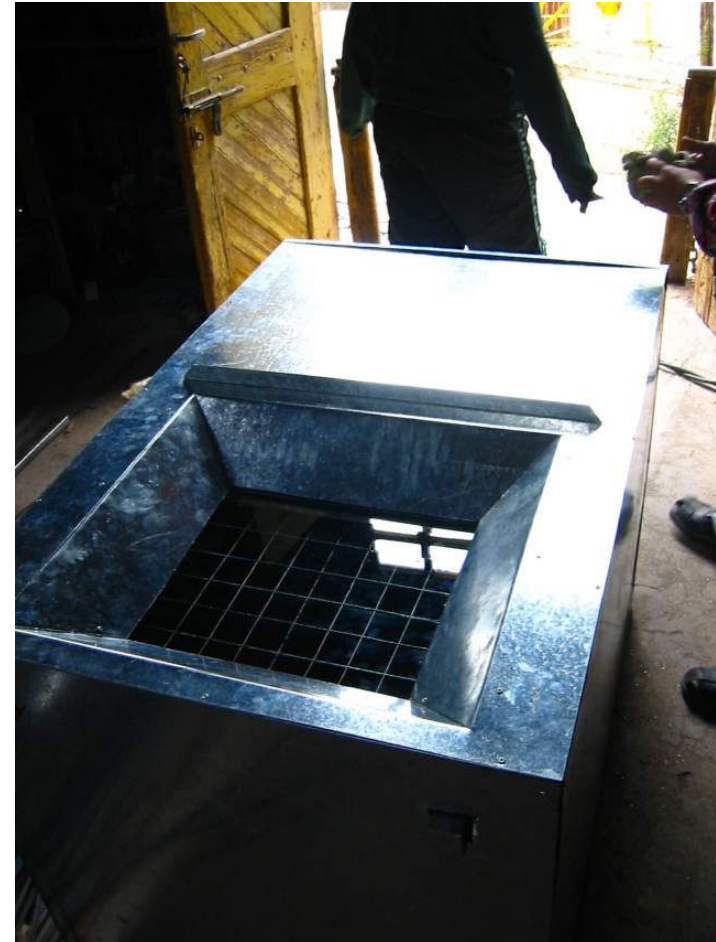
Finally the cover is placed on the box and is riveted.
