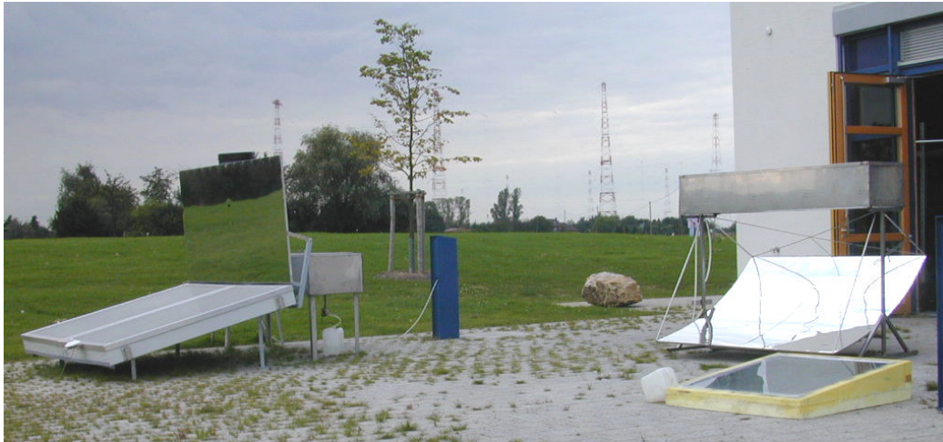
Fig. 2: Greenhouse-type still in comparison with desalination units with flat plate collector and parabolic reflector
