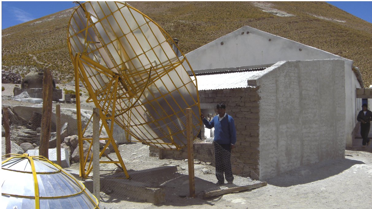
Fig.2: Solar community oven powered by Scheffler reflector
