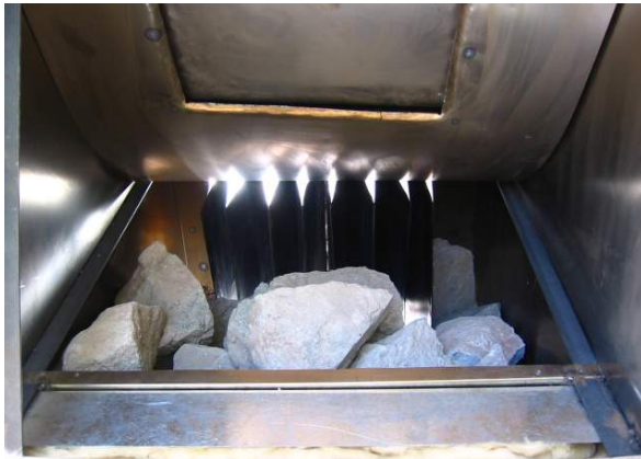
Fig.5: Zic-zac receiver and pebblebed storage
