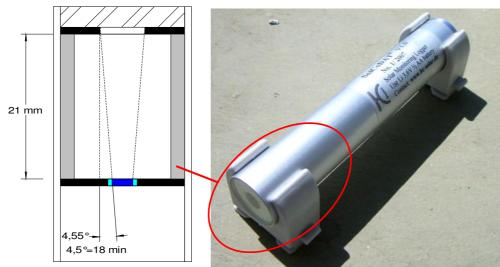
Fig. 1: Schematic of orifice and photo of SolCoDat
